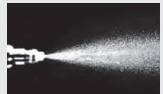
Injector spray pattern after P.i. treatment.
